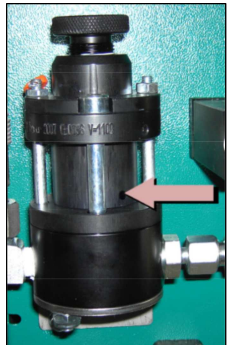
Figure 1: Position for oil refill
