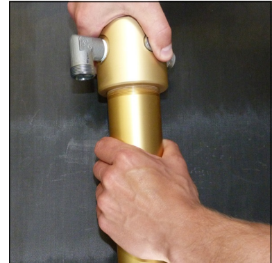
Fig. 1 - Unscrew and remove filter top
