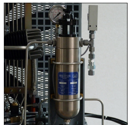
Oil / water separators final stage
