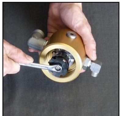
Fig. 2 - Loose nut at the separator top
