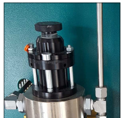
Safety valve 4th stage
