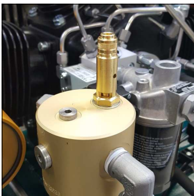
Safety valve 1st stage
