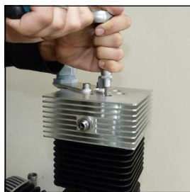
Fig. 1 - Loose valve head screws
