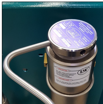
Fig. 2 - Unscrew the filter housing cover.
