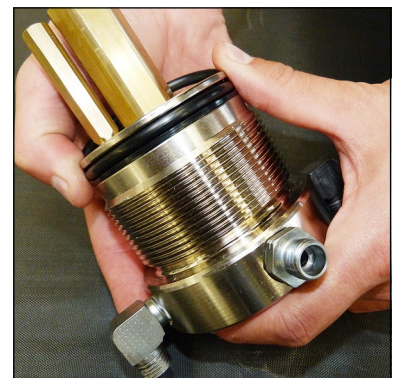
Fig. 4 - Change o-ring and back-up rings
