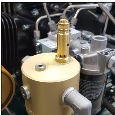
Safety valve 1st stage
