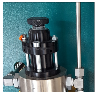
Safety valve 4th stage
