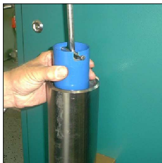
Fig. 4 - Pull the cartridge out of the housing.
