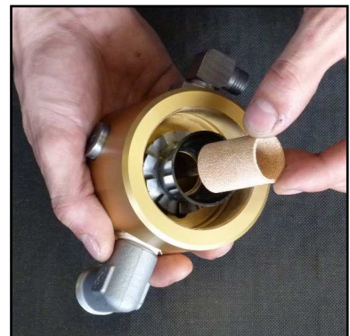
Fig. 3 - Change sinter filter
