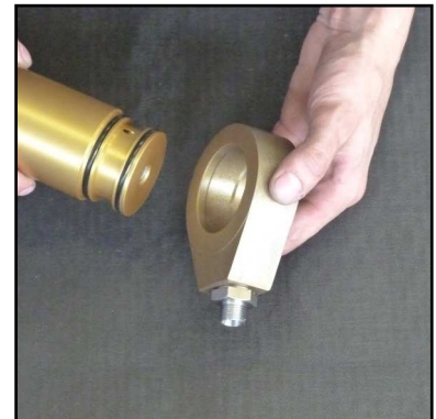
Abb. 6 - Remove the base ring
