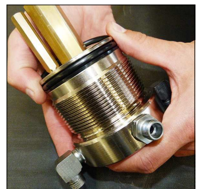
Fig. 4 - Change o-ring and back-up rings
