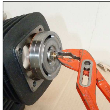
Fig. 2 - Pull out inlet and outlet valve
