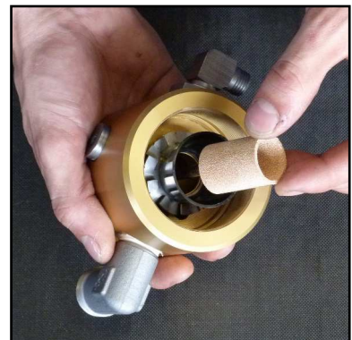
Fig. 3 - Change sinter filter
