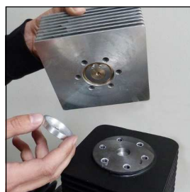
Fig. 2 - Remove lower valve gasket
