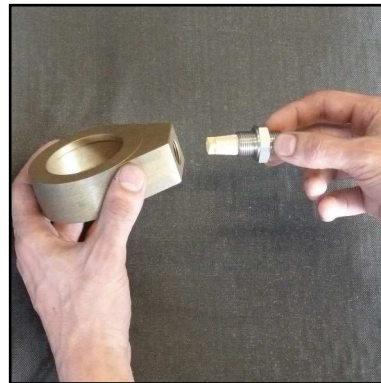
Abb. 8 - Change sinter filter
