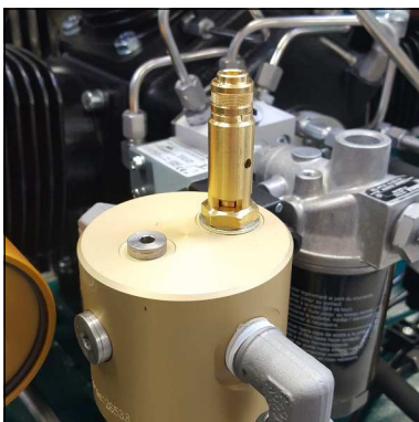
Safety valve 1st stage
