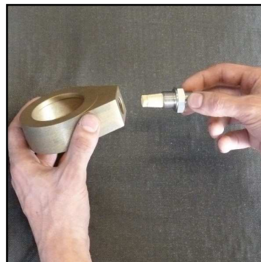
Abb. 8 - Change sinter filter
