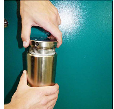
Fig. 1 - Open Filter cover
