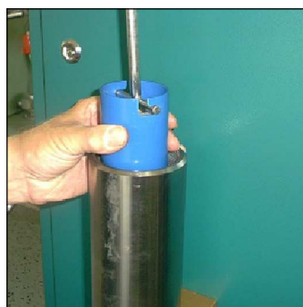
Fig. 4 - Pull the cartridge out of the housing.
