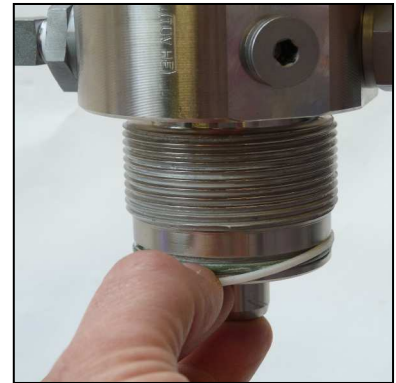
Fig. 1 - Change o-ring and back-up ring
