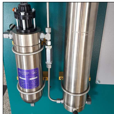
Fig. 3 - Loose pipe connections and nuts
