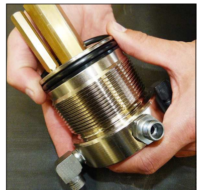
Fig. 4 - Change o-ring and back-up rings
