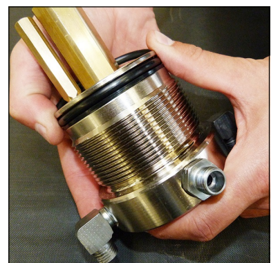
Fig. 4 - Change o-ring and back-up rings
