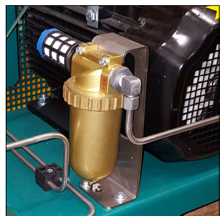
Oil / water separators final stage
