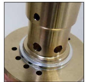
Fig. 4 - Ensure correct mounting position of the upper valve gasket
