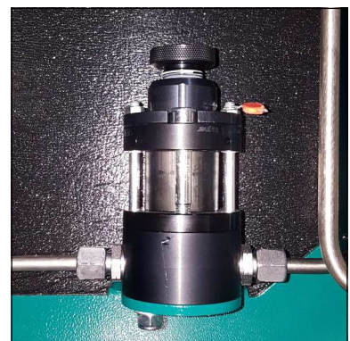
Safety valve 4th stage
