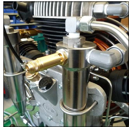
Safety valve 1st stage
