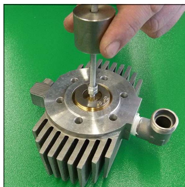
Fig. 4 - Remove inlet and outlet valve
