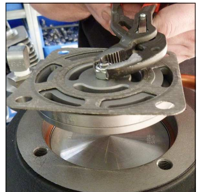
Fig. 2 - Pull out inlet and outlet valve
