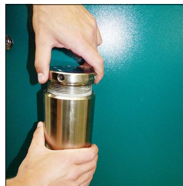
Fig. 1 - Open Filter cover
