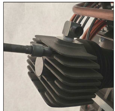
Fig. 2 - Loosen valve head screws
