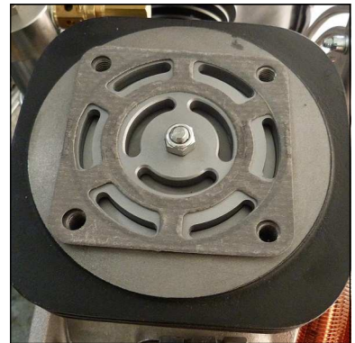
Fig. 4 - Place and align upper valve gasket
