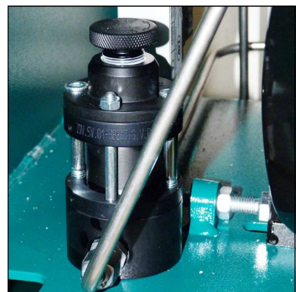
Safety valve 3rd stage
