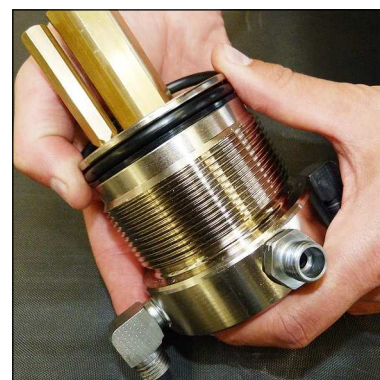
Fig. 4 - Change o-ring and back-up rings
