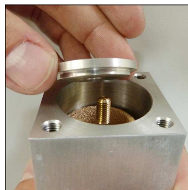
Fig. 5 - Place filter washer and washer
