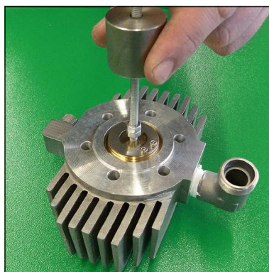
Fig. 4 - Remove inlet and outlet valve
