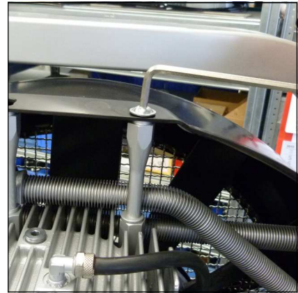
Fig. 1 - Remove top mounting screws
