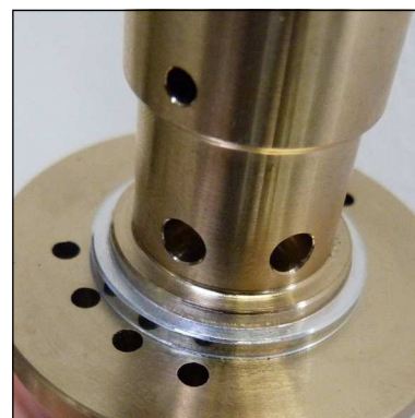
Fig. 5 - Ensure correct mounting position of the upper valve gasket
