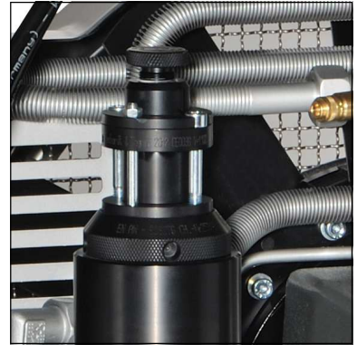
Fig. 1 - Remove/screw in filter cover
