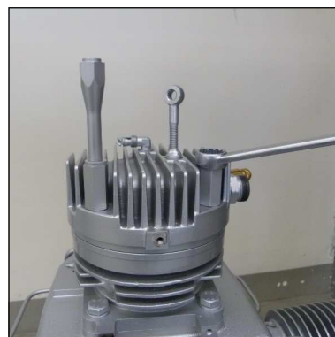
Fig. 6 - Remove special hexagon bolt
