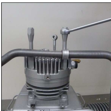
Fig. 5 - Remove cooling pipe bracket
