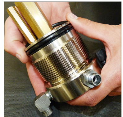
Fig. 4 - Change o-ring and back-up rings
