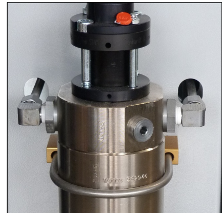
Fig. 1 - Loosen pipe connections and mounting screws
