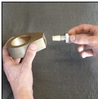
Abb. 7 - Change sinter filter
