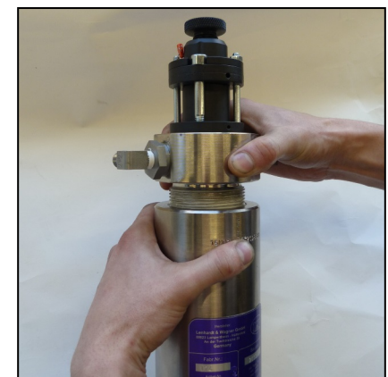
Fig. 3 - Open pre-filter cover
