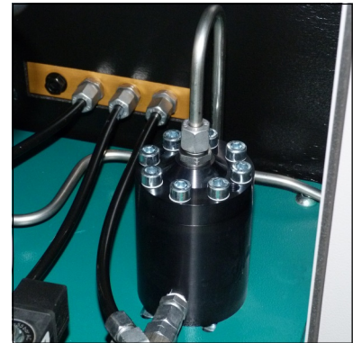
Fig. 1 - Condensate stop valve housing
