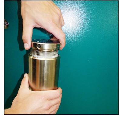
Fig. 1 - Open Filter cover
