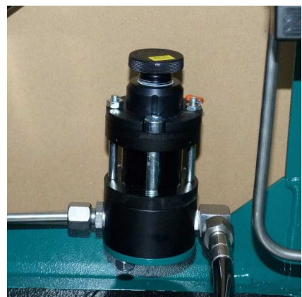
Safety valve 3rd stage
