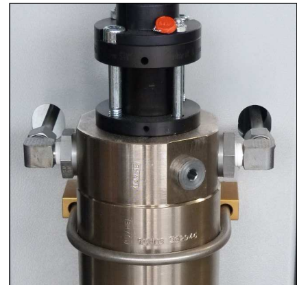
Fig. 1 - Loosen pipe connections and mounting screws
