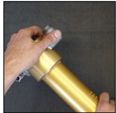
Fig. 1 - Unscrew and remove filter top
