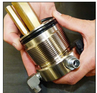
Fig. 4 - Change o-ring and back-up rings
