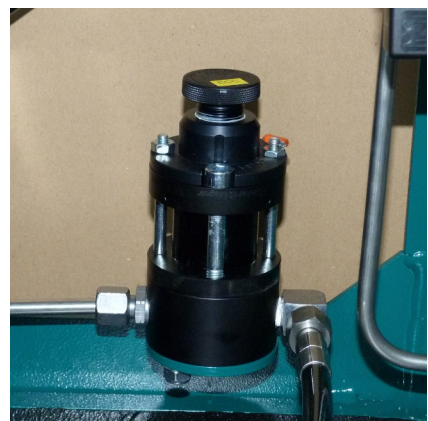
Safety valve 3rd stage
