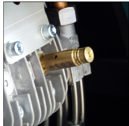
Safety valve 2nd stage
