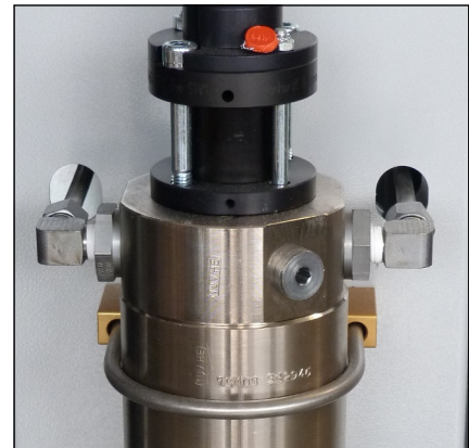
Fig. 1 - Loosen pipe connections and mounting screws
