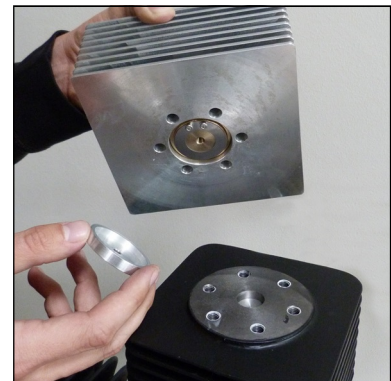
Fig. 2 - Remove lower valve gasket
