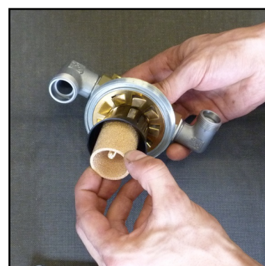
Fig. 3 - Change sinter filter
