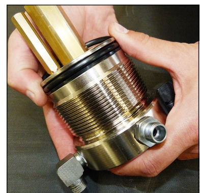
Fig. 4 - Change o-ring and back-up rings
