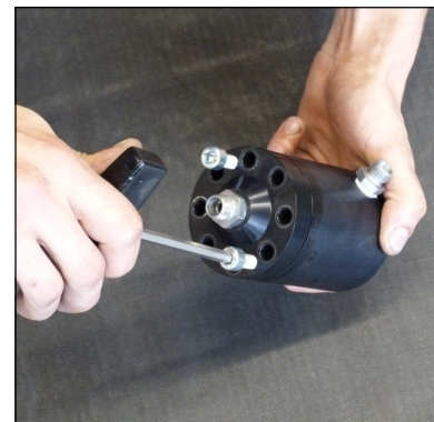
Fig. 2 - Remove the cover
