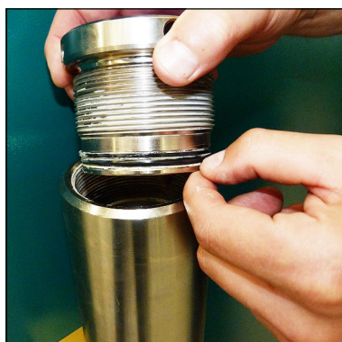
Fig. 2 - Change o-ring and back-up rings
