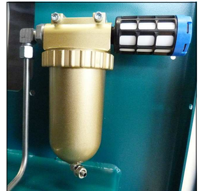
Oil / water separators final stage
