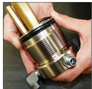
Fig. 4 - Change o-ring and back-up rings
