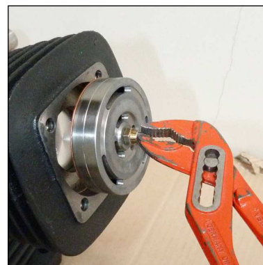
Fig. 2 - Pull out inlet and outlet valve
