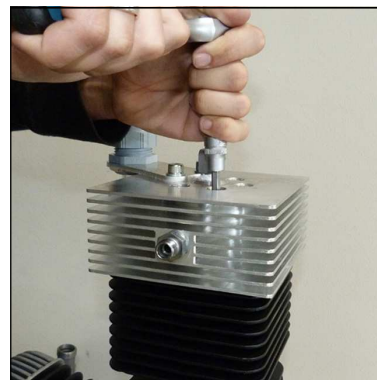
Fig. 1 - Loosen valve head screws
