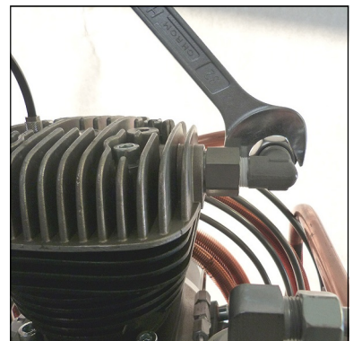
Fig. 6 - Connect pipe connections and tighten
