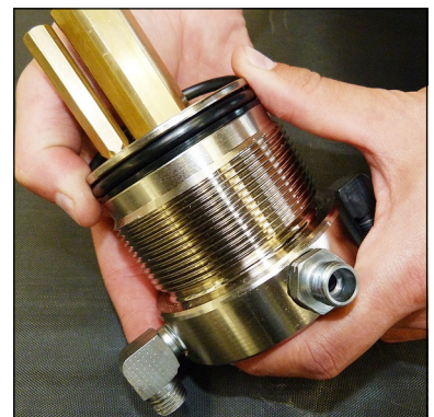
Fig. 4 - Change o-ring and back-up rings
