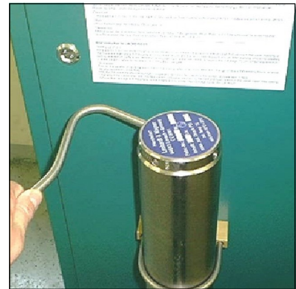
Fig. 1 - Unscrew the filter housing cover.
