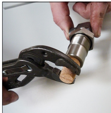
Fig. 3 - Change sinter filter
