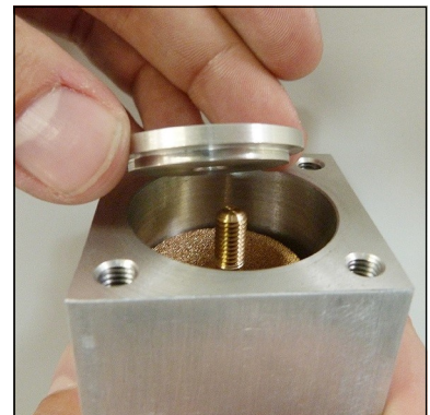
Fig. 5 - Place filter washer and washer
