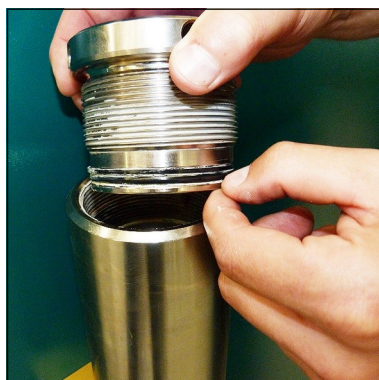
Fig. 2 - Change o-ring and back-up rings
