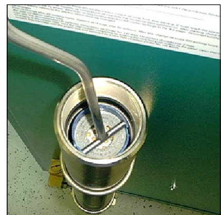
Fig. 2 - Place the T-piece end of the filter key in the top of the filter cartridge.
