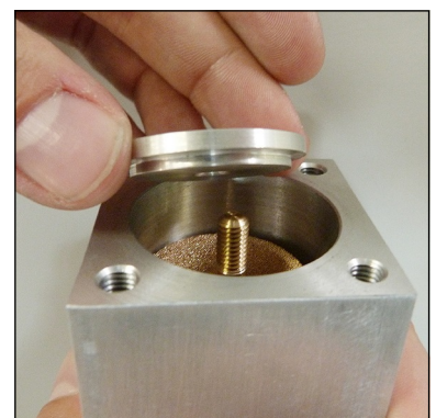
Fig. 5 - Place filter washer and washer
