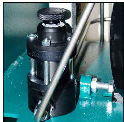
Safety valve 3rd stage
