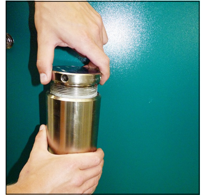
Fig. 1 - Open Filter cover
