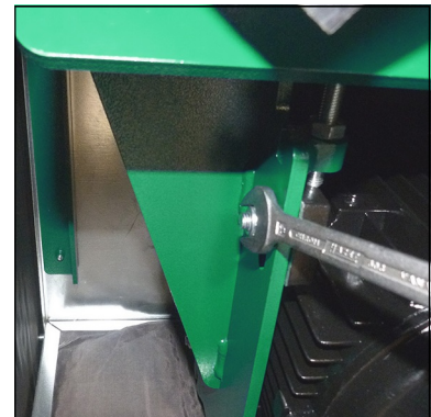
Fig. 1 - Loosen mounting screws
