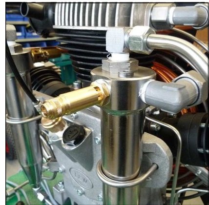
Safety valve 1st stage
