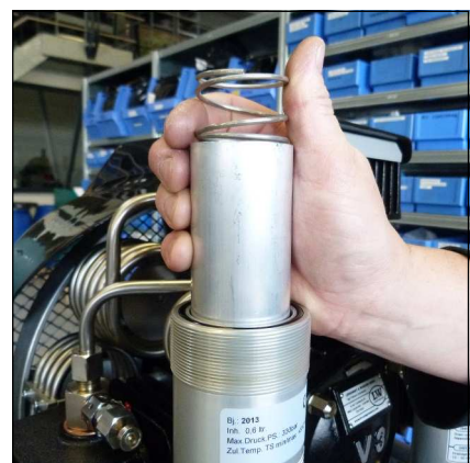
Fig. 3 - Filter cartridge and spring
