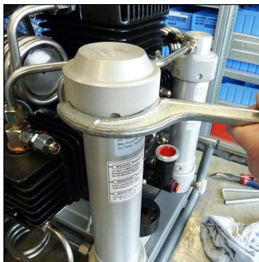
Abb. 1 - Open filter cover
