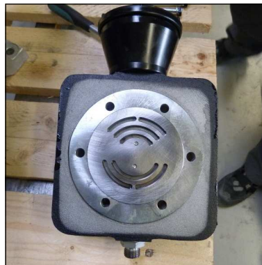
Fig. 3 - Correct position of in-and outlet valve
