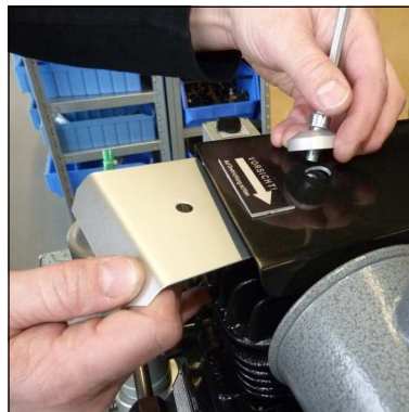
Fig. 2 - Remove protection plate
