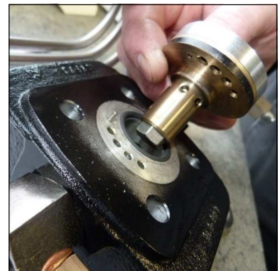
Fig. 4 - Ensure correct valve position (centre pin)
