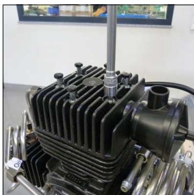
Fig. 5 - Valve head screws
