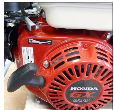
Fig. 2 - Speed control and pull start
