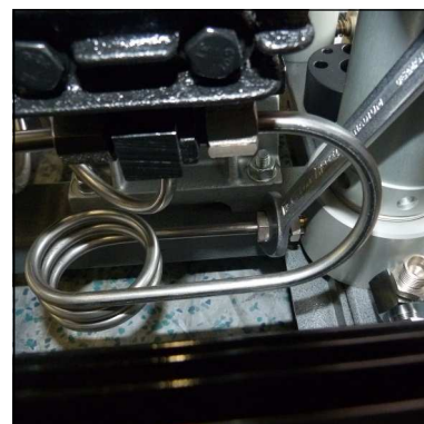
Fig. 2 - Loosen pipe connections of the filter housing
