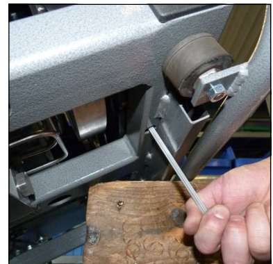
Fig. 3 - Loosen both bottom mounting screws
