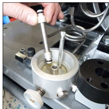
Abb. 5 - Remove duct collar and change o-rings
