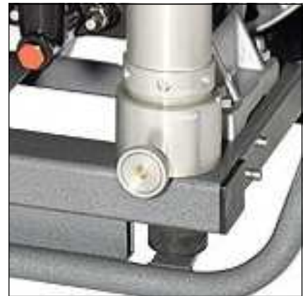
Fig. 1 - Condensate drain valve 2nd stage
