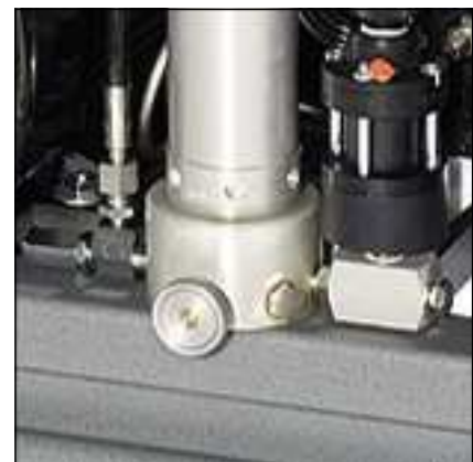
Fig. 2 - Oil- / water separator 3rd stage
