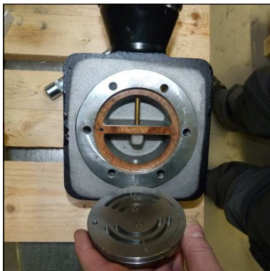
Fig. 2 - Correct position of in-and outlet valve
