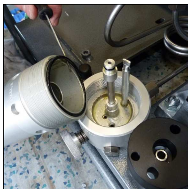
Abb. 4 - Remove lock ring
