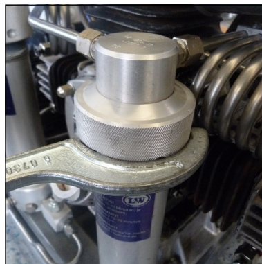
Fig. 5 - Tighten lock ring
