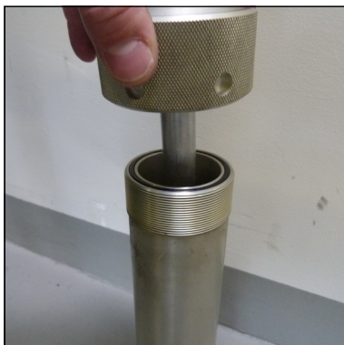
Fig. 4 - Remove lock ring and change o-ring
