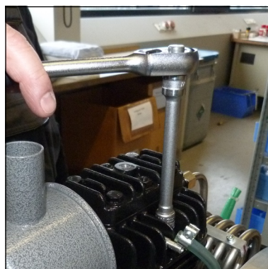
Fig. 6 - Tighten valve head
