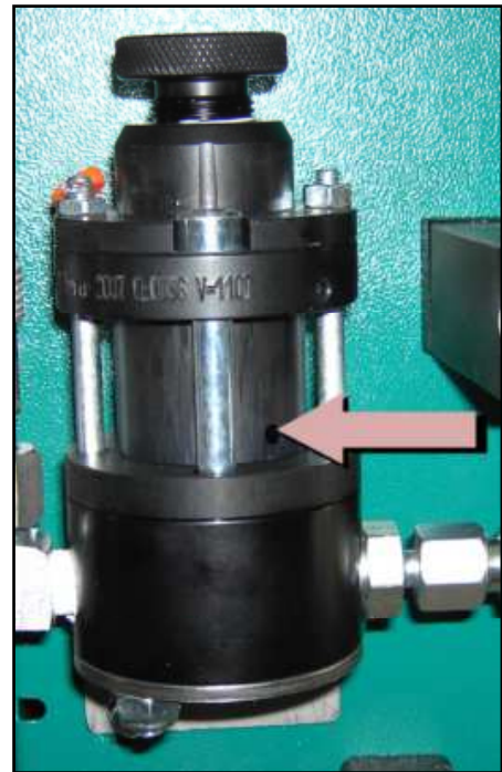
Figure 1: Position for oil refill
