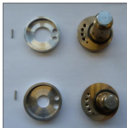
Fig. 2 - In – and outlet valve c/w gaskets 2nd stage (top) and 3rd stage (below)
