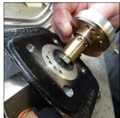
Fig. 4 - Ensure correct valve position (centre pin)
