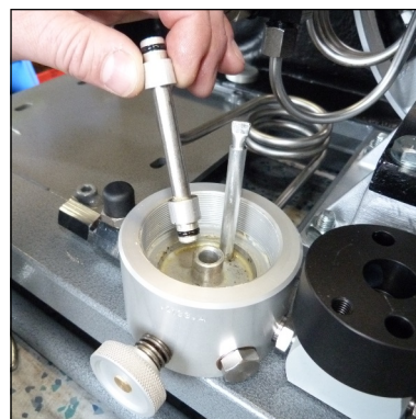
Fig. 5 - Remove duct collar and change o-rings
