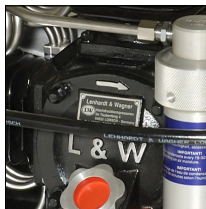
Rotation direction arrow on the compressor block
