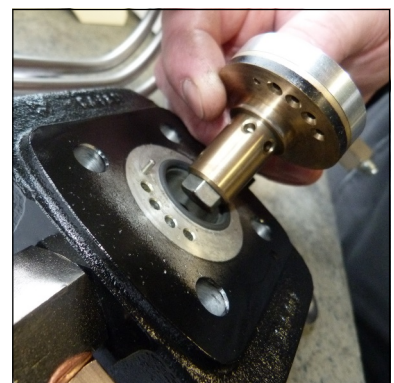
Fig. 5 - Ensure correct valve position (centre pin)
