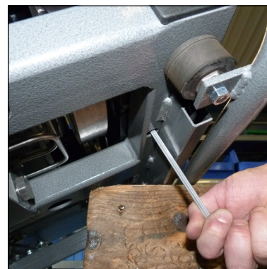
Fig. 3 - Loosen both bottom mounting screws
