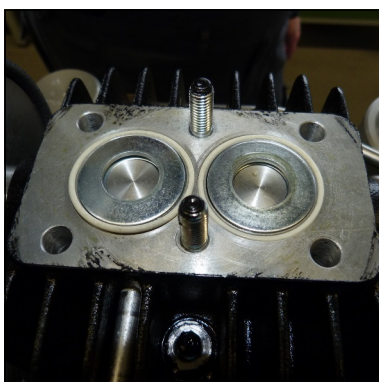
Fig. 5 - Spring plate inside the valve head
