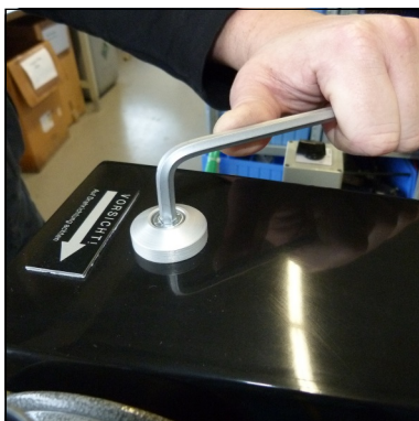
Fig. 1 - Remove top mounting screws
