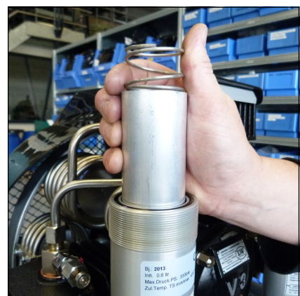
Fig. 3 - Filter cartridge and spring
