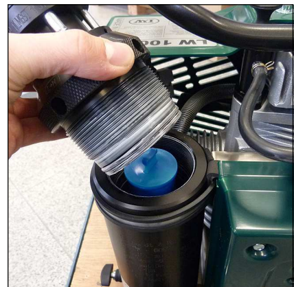
Fig. 2 - Remove filter housing cover
