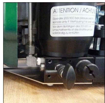
Fig. 2 - Condensate drain valve 3rd.stage
