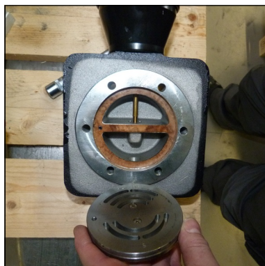
Fig. 2 - Correct position of in-and outlet valve
