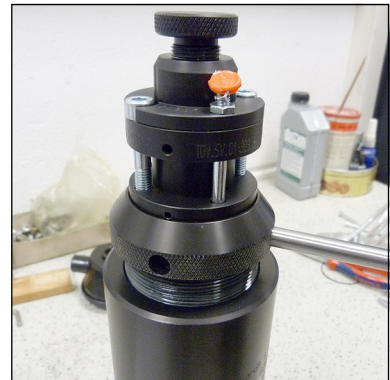
Fig. 1 - Remove/screw in filter cover
