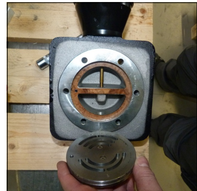
Fig. 5 - Remove in- and outlet valve
