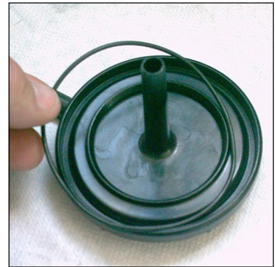
Fig. 3 - Place o-ring into the filter housing
