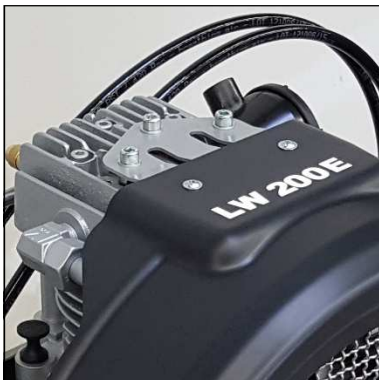
Fig. 1 - Loosen mounting screws of the fan protection cover
