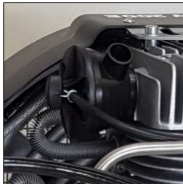
Fig. 2 - Remove spring wire clamp
