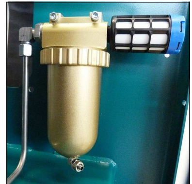
Oil / water separators final stage
