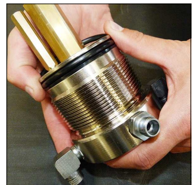
Fig. 4 - Change o-ring and back-up rings
