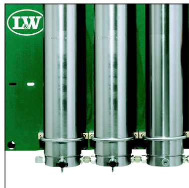
Fig. 3 - Loosen u-clamps and pipe connections
