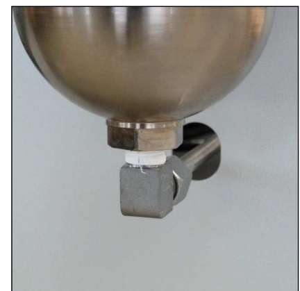
Fig. 2 - Loosen pipe connections and mounting screws
