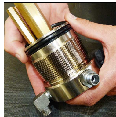
Fig. 4 - Change o-ring and back-up rings
