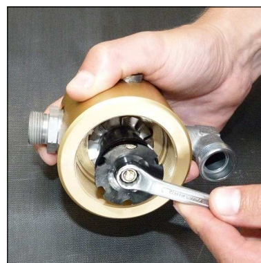
Fig. 1 - Loosen nut at the separator top
