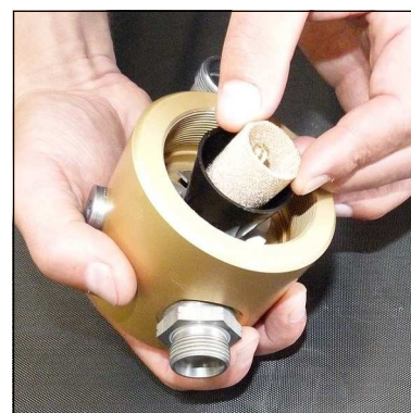
Fig. 2 - Change sinter filter
